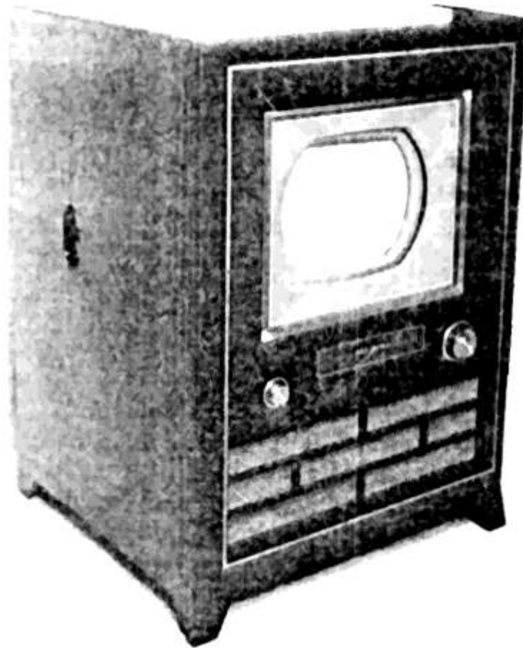
Fig. 1—The CT-100 color television receiver.
